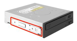
**4.** Press the ODD rail onto both side of the ODD.
